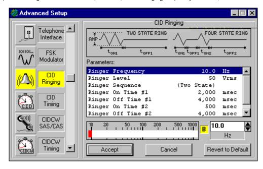
2) Start a Caller ID transmission by either clicking on the "Start" icon or by pressing the F5 key. During the ringing cycle, record the level of the signal in the table below. If the ringing time is not long enough for an accurate measurement, then increase the Ringer On Time #1 in the Advanced Setup window. Repeat this procedure with all of the other frequencies shown in the table.
