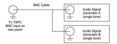
Note: If a dual tone signal generator is available, then the second generator is not required
